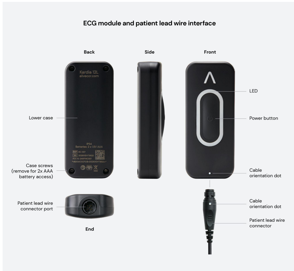
Figure 1: ECG Module and Patient Lead Wire Interface
